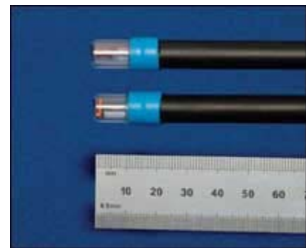
FIGURE 2. The axial and transverse telecoil probes.
