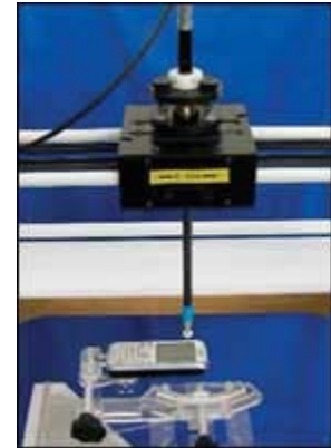
FIGURE 3. 2-D scan with an E-field probe (wireless device at bottom).
