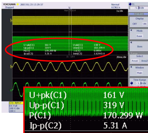
Fig 17 Example of measurement and computation by DL9000
