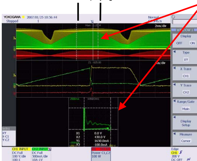
Fig 13 Example of ASO measurement by DL9000
