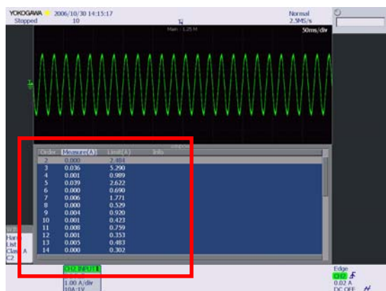
The actual measured value of each harmonic order is displayed along with the limit values, and any data exceeding the limit is marked.
